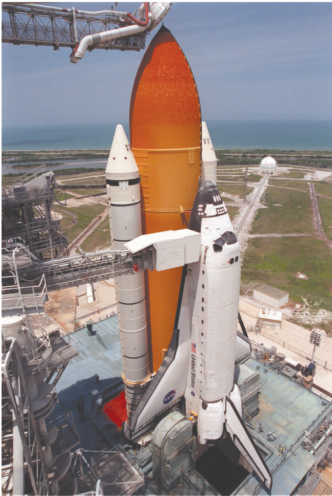
With the Shuttle on the pad, the Orbiter Access Arm and White Room is extended to the cockpit entry. Above the orange external tank is the "beanie cap" or vent hood.
