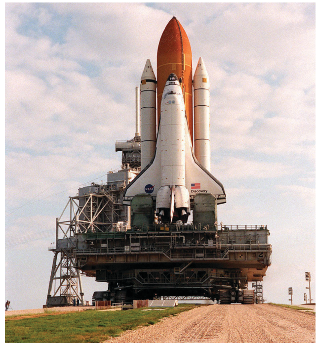
The Shuttle atop the Mobile Launcher Platform moves to the pad via the crawler transporter beneath.
