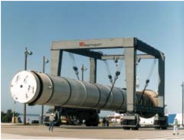
A spent SRB is lifted in a hoisting slip in the Hangar AF area at CCAFS. It will be washed down and moved to the Hangar.
