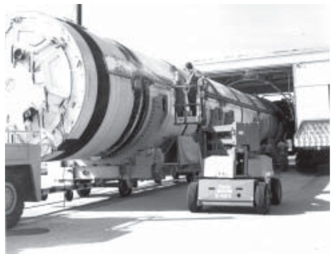
After retrieval post-launch, an SRB is processed through the washing station at Hangar AF.
