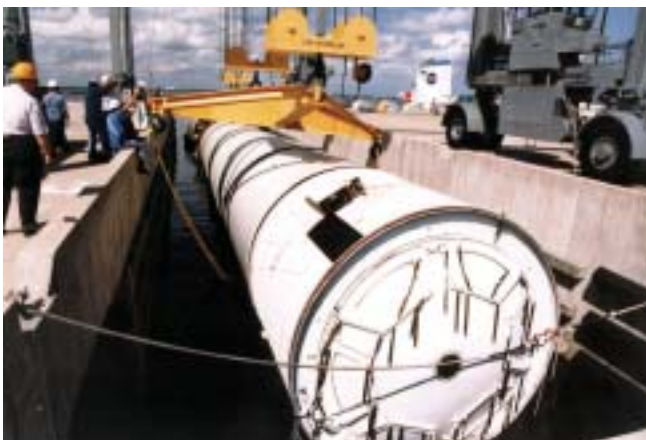
Workers at CCAFS help maneuver the SRB into the hoisting sling.
