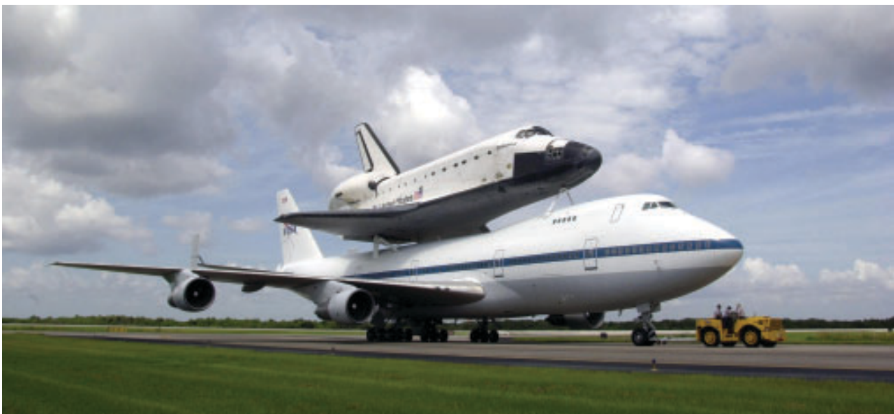
Space Shuttle Endeavour is towed toward the Mate-Demate Device following landing on runway 15 at KSC's Shuttle Landing Facility atop a modified Boeing 747 Shuttle Carrier Aircraft.
