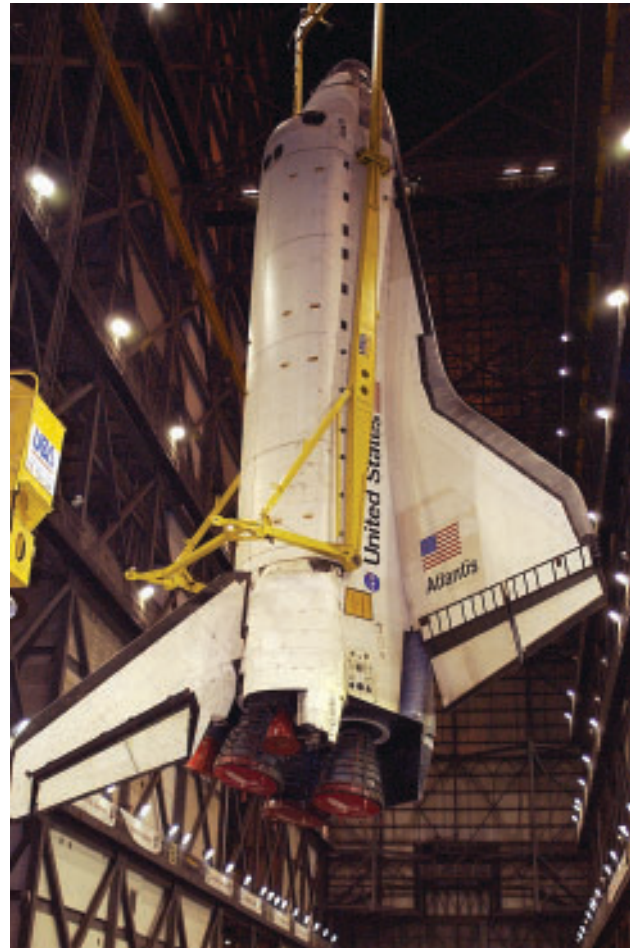
A huge crane in the Vehicle Assembly Building is used to lower or raise an orbiter into position for stacking or destacking.
