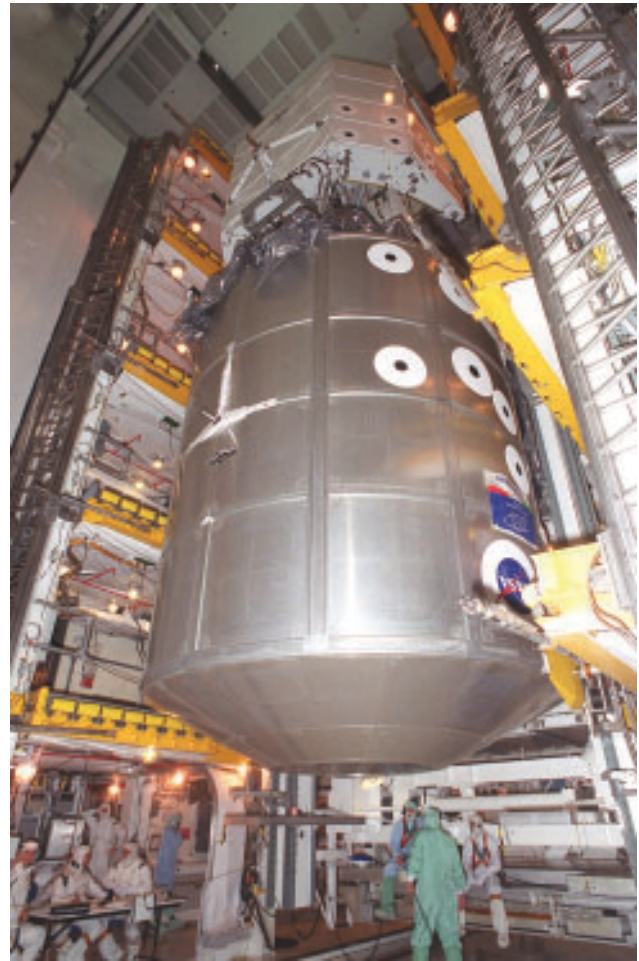
Two payloads in the Canadian robotic arm or Space Station Remote Manipulator System, and the Multi-Purpose Logistics Module Raffaello in are moved into the Payload Changeout Room for mission STS-100.
