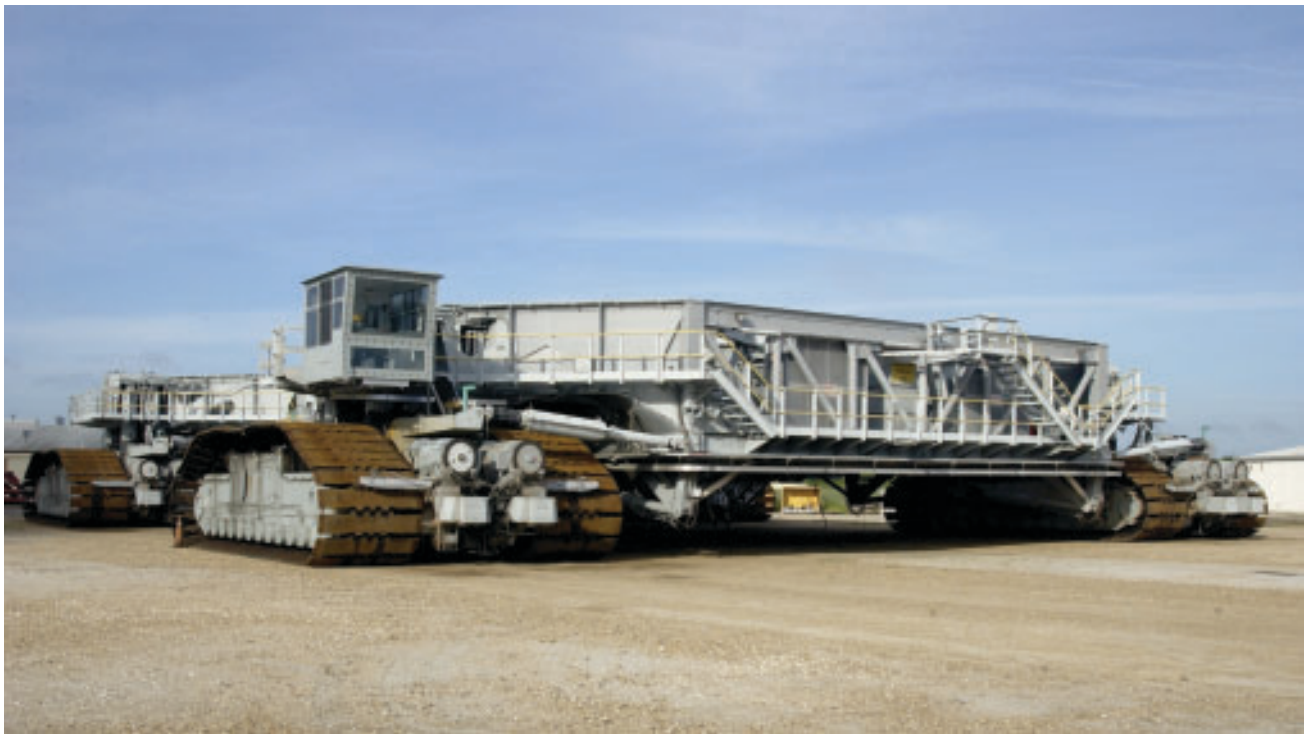
The Crawler-Transporter (6 million pounds) can lift the Space Shuttle on its Mobile Launcher Platform (combined weight about 11 million pounds) and move it to and from the launch pads. A Crawler has eight tracks, each of which has 57 shoes or cleats, each weighing approximately one ton.
