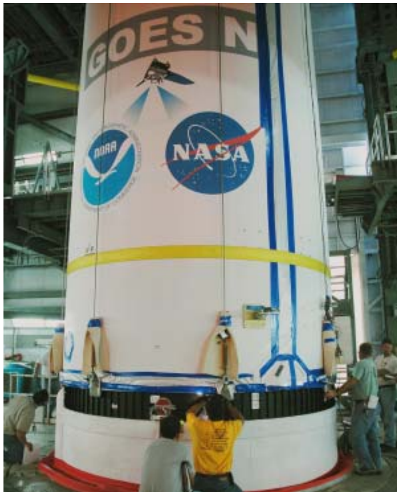
IN THE mobile service tower on Launch Complex 37 at Cape Canaveral Air Force Station, workers check the attach points on the GOES-N spacecraft and Boeing Delta IV rocket.
