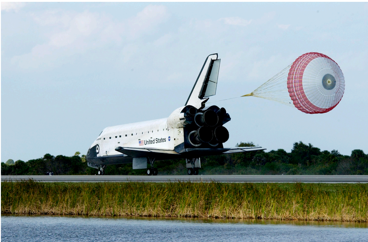
Space Shuttle Endeavour's drag chute slows down the orbiter as it lands on runway 33 at the SLF.
