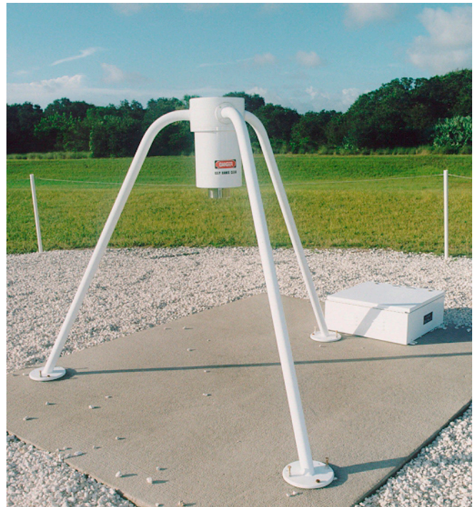
One of the 31 electric field mills that compose the Launch Pad Lightning Warning System. They are called mills because they have a rotating, four-bladed shield much like arms of a windmill. The shield contained in the bottom of the round housing alternately exposes and covers metal sensing plates, resulting in an alternating current proportional to the atmospheric electric field.
