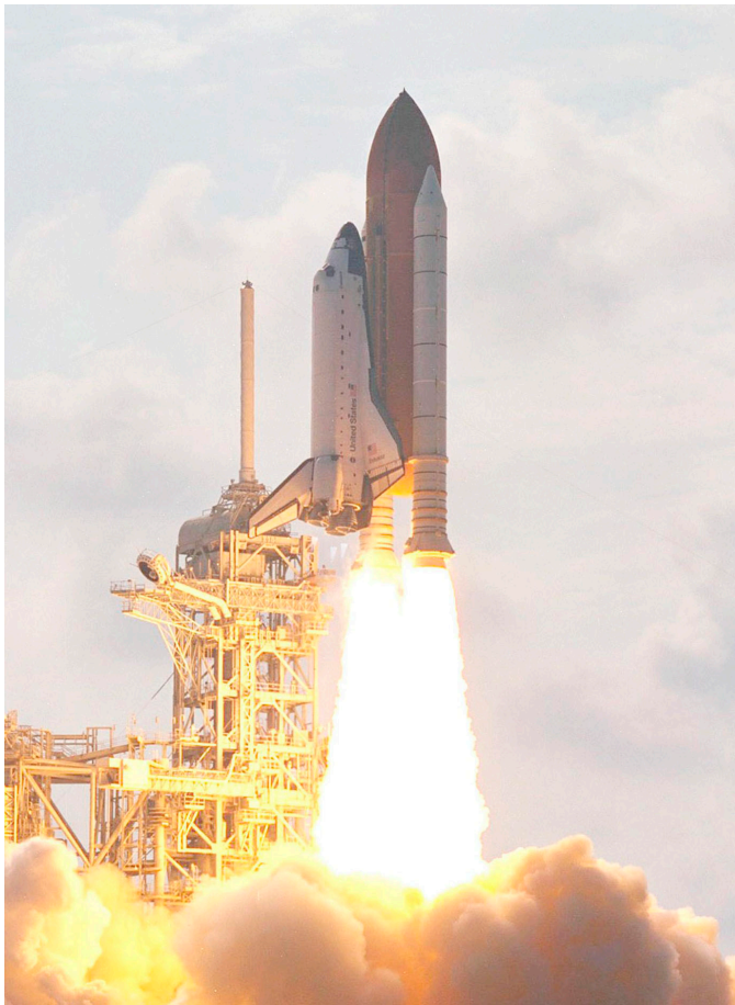
Space Shuttle Endeavour clears the lightning mast and attached catenary wire as it hurtles into space on mission STS-111 to the International Space Station June 5, 2002. The mast and wire provide the primary lightning protection system for the orbiter while it is on the pad. Mission STS-111 is the 18th flight of Endeavour and the 110th flight overall in NASA's space shuttle program.
