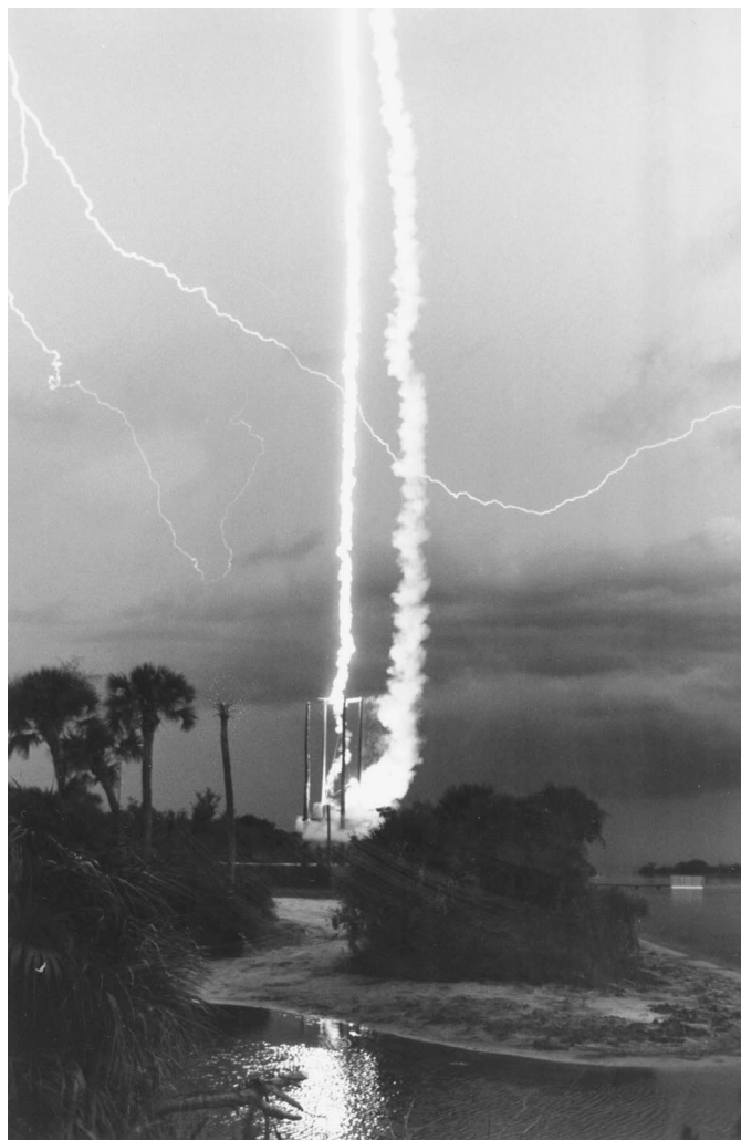
The lightning event begins when lightning strikes the rocket, launched from the Rocket Triggered Lightning launch pad at Kennedy Space Center, and the 3,000-foot copper wire being trailed from the rocket. The wire is then vaporized as it follows the path to a lightning rod attached to the instrumented launcher. As the wire burn dissipates, it creates an effect called “rosary bead lightning.” This can be the prelude to natural lightning restrikes. The initiation of a wire burn can also induce natural intercloud lightning during the event, as seen in this sequence.
