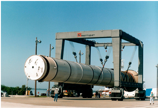
A spent SRB is lifted in a hoisting slip in the Hangar AF area at CCAFS. It will be washed down and moved to the hangar.
