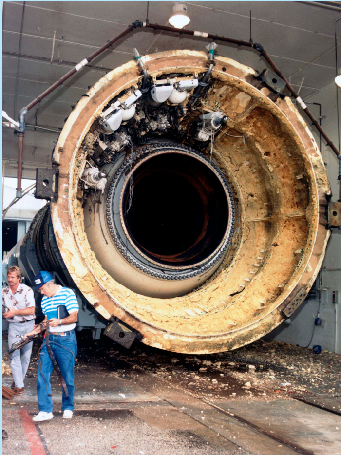
(Left) The segment is in the west wash area at Hangar AF, CCAFS, on a rail car dolly prior to SRB aft skirt demating. Residual aft skirt foam can be seen.
