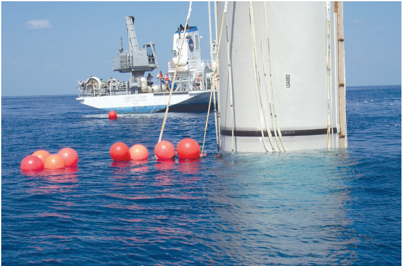
A Solid Rocket Booster Retrieval Ship has arrived on scene after splashdown of an SRB segment following a space shuttle launch. The segment floats vertically until divers can insert an enhanced diver-operated plug (EDOP) into the nozzle of the booster. The EDOP pumps air into the empty casing until all water is expelled and it falls horizontally and can be towed back to port.
