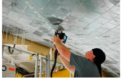
In Orbiter Processing Facility bay 1 at NASA's Kennedy Space Center, a United Space Alliance technician uses a laser tool to take step and gap measurements on Thermal Protection System tiles on the underside of orbiter Atlantis.
