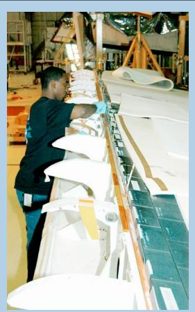
In the Orbiter Processing Facility, a technician prepares the blanket insulation to be installed on the body flap on orbiter Discovery. The blankets are part of the Orbiter Thermal Protection System's, thermal shields to protect against temperatures as high as 3,000° Fahrenheit, which are produced during descent for landing.
