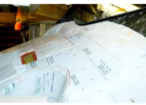
A gap test is being performed on the tiles below the windshield on the orbiter Atlantis.
