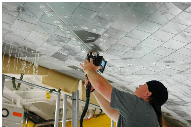
In Orbiter Processing Facility bay 1 at NASA's Kennedy Space Center, a United Space Alliance technician uses a laser tool to take step and gap measurements on Thermal Protection System tiles on the underside of orbiter Atlantis.
