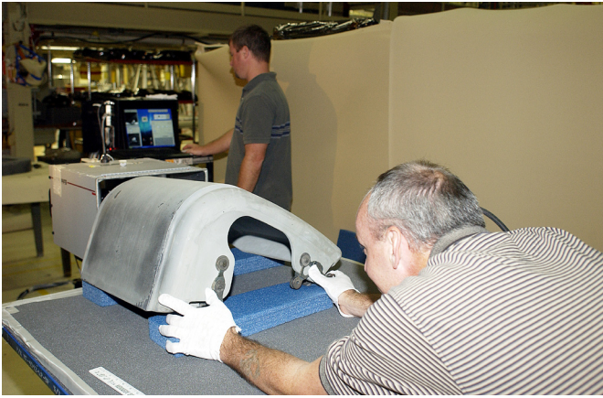
In the Orbiter Processing Facility, a United Space Alliance worker positions a reinforced-carbon carbon panel on the table to perform flash thermography.
