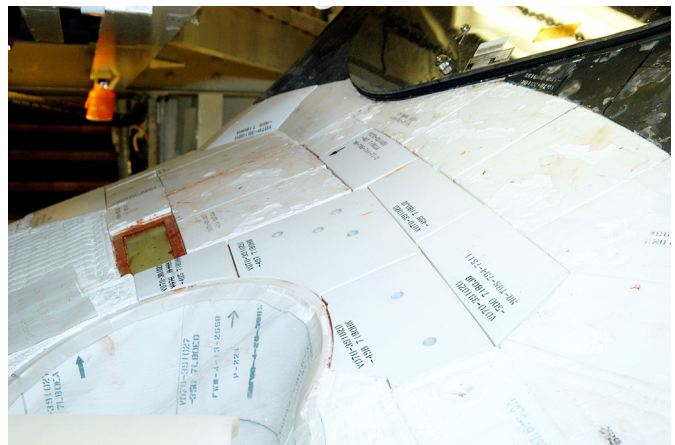
A gap test is being performed on the tiles below the windshield on the orbiter Atlantis.
