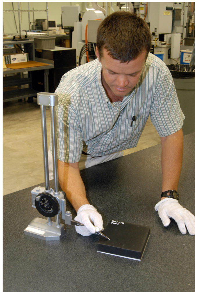
In the Thermal Protection System Facility, Tim Wright, engineering manager with United Space Alliance, tests a new tile, called “Boeing replacement insulation” or “BRI-18.” The new tiles have replaced older tiles around main landing gear doors, external tank doors and nose landing gear doors.
