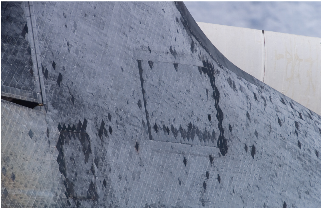
During a backflip maneuver during the STS-120 mission, the underside of the space shuttle Discovery is featured in this image photographed by an Expedition 16 crewmember. Visible are a landing gear door (large square at center) and an external tank umbilical door (lower left).
