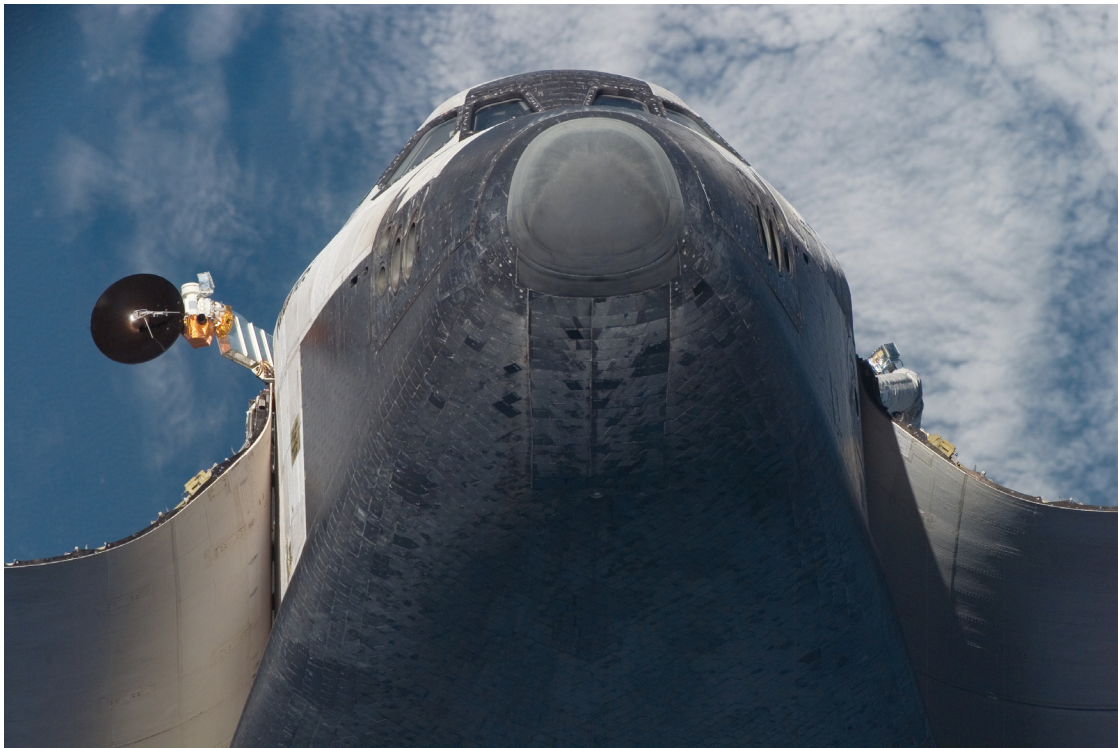
A low-angle view of the nose and underside of the Space Shuttle Atlantis' crew cabin was provided by Expedition 16 crewmembers. Before docking with the International Space Station, STS-122 Commander Steve Frick flew the shuttle through a roll-pitch maneuver, or basically a backflip, to allow the space station crew a good view of Atlantis' heat shield.
