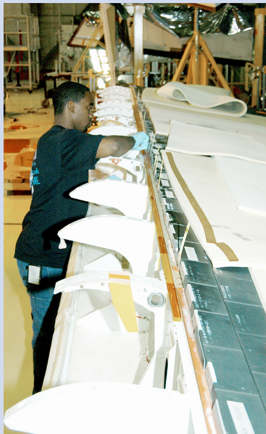
In the Orbiter Processing Facility, a technician prepares the blanket insulation to be installed on the body flap on orbiter Discovery. The blankets are part of the Orbiter Thermal Protection System's, thermal shields to protect against temperatures as high as 3,000° Fahrenheit, which are produced during descent for landing.
