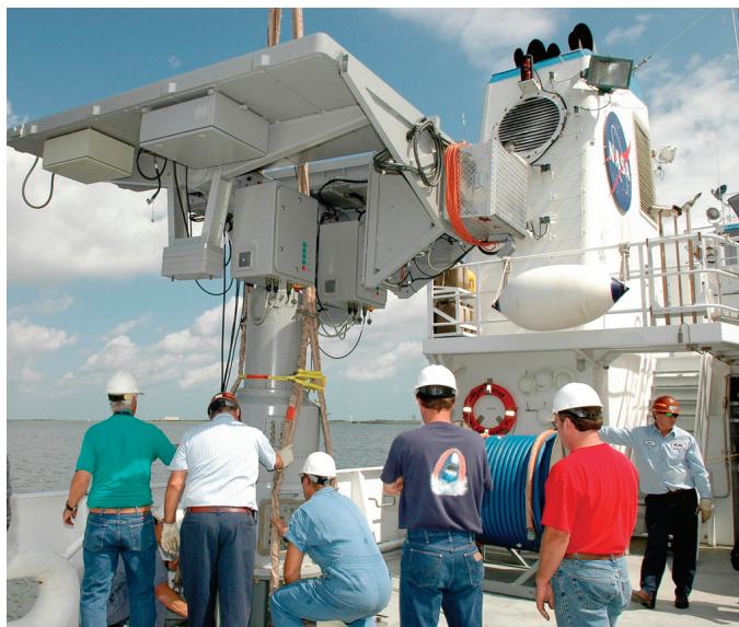
At Hangar AF at Cape Canaveral Air Force Station, workers on the Liberty Star, one of the two SRB Retrieval Ships, oversee the safe placement of an X-band Doppler radar array onto the deck. The radar will be used for tracking support on NASA's Return to Flight mission, STS-114, on Space Shuttle Discovery.
