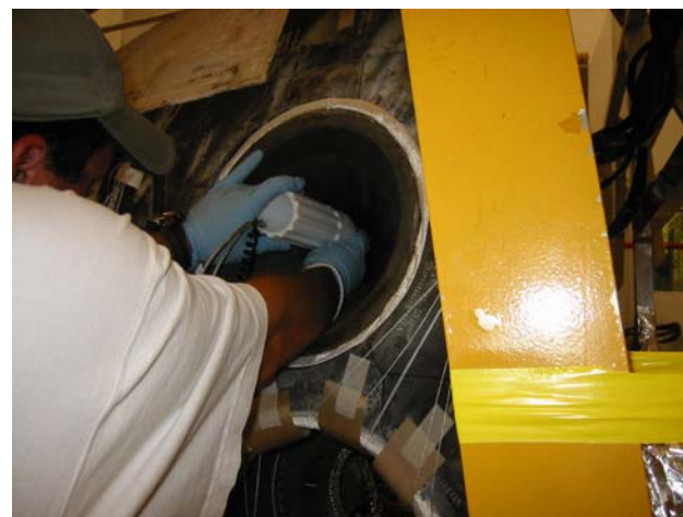
QUALITY ASSURANCE inspector James Allen Atwell is using the fuel hole inspection device to look into a nozzle in the Orbiter Processing Facility bay 2.
