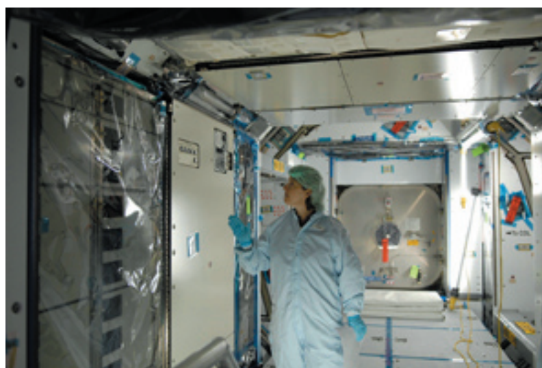
STS-120 Commander Pam Melroy checks out the Harmony module during a crew equipment interface test. The module is 23.6 feet long and 4.5 feet in diameter. Its pressurized volume is 2,666 cubic feet.
