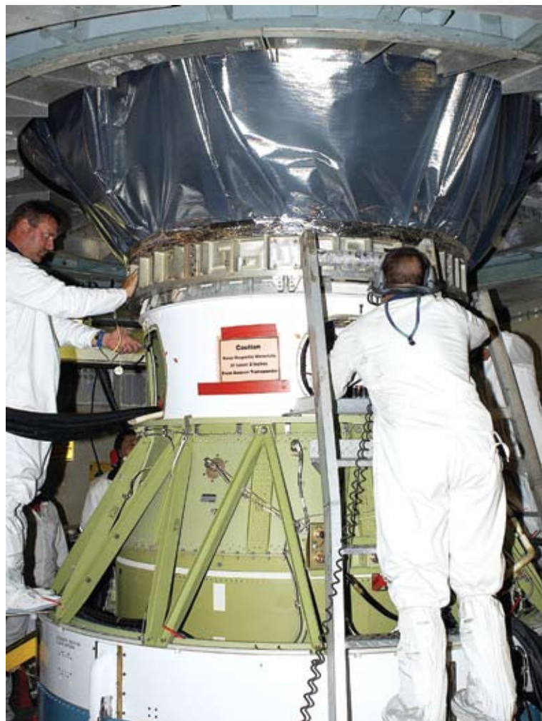
Workers on Launch Pad 17-B, Cape Canaveral Air Force Station, complete mating of the Mars Exploration Rover 1 (MER-B) above, to the Boeing Delta rocket below. The second of twin rovers sent to Mars, it is equipped with a robotic arm, a drilling tool, three spectrometers, and four pairs of cameras that allow it to have a human-like, 3-D view of the terrain. The rovers landed safely on Mars in 2004 and lasted much longer than the three months originally planned for. They provided spectacular views and data that is still being analyzed.
