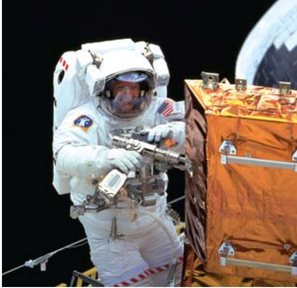
On a Hubble Servicing Mission (STS-103) in 1999, astronaut Claude Nicollier, mission specialist from the European Space Agency, works at a storage enclosure, using one of the Hubble power tools, during the second of three extravehicular activities.
