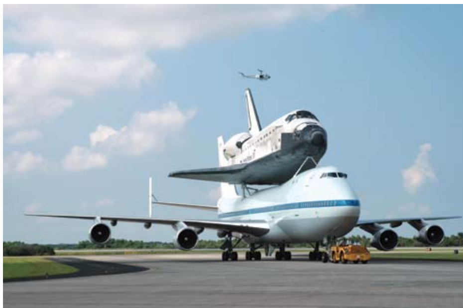
Space Shuttle Discovery, atop a modified Boeing 747 Shuttle Carrier Aircraft, is towed to the mate/demate device at NASA Kennedy Space Center's Shuttle Landing Facility following touchdown on runway 15 on Aug. 21, 2005. The cross-country ferry flight became necessary when two days of unfavorable weather conditions at KSC forced Discovery to land at Edwards Air Force Base, California, on Aug. 9 following mission STS-114.
