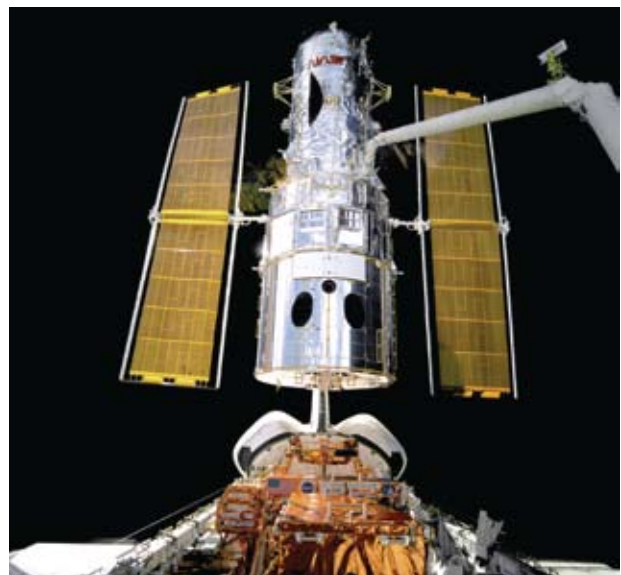
Discovery's robot arm lifts the Hubble Space Telescope out of the payload bay after a successful servicing mission, STS-103, in December 1999.
