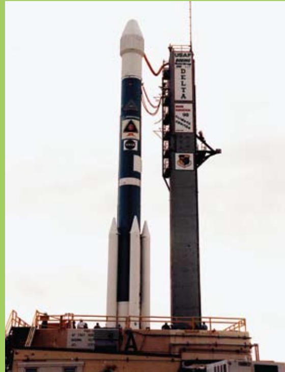
Protected by its gantry, a Delta rocket awaits launch under leaden skies at Complex 17. It later hurled a GOES weather satellite into a geostationary orbit. Three of the Delta's five strap-on solid rocket boosters are visible in this photo.
