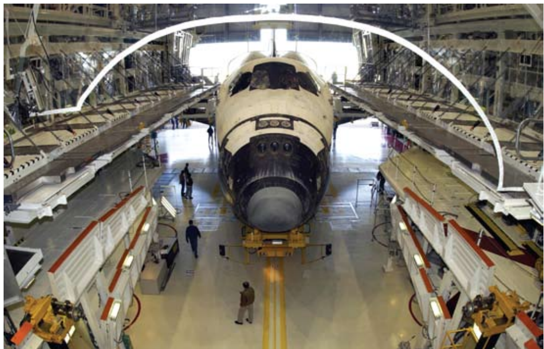
Orbiter Atlantis begins backing out of the Orbiter Processing Facility for rollover to the Vehicle Assembly Building, where it will be mated with the external tank and solid rocket boosters for launch.
