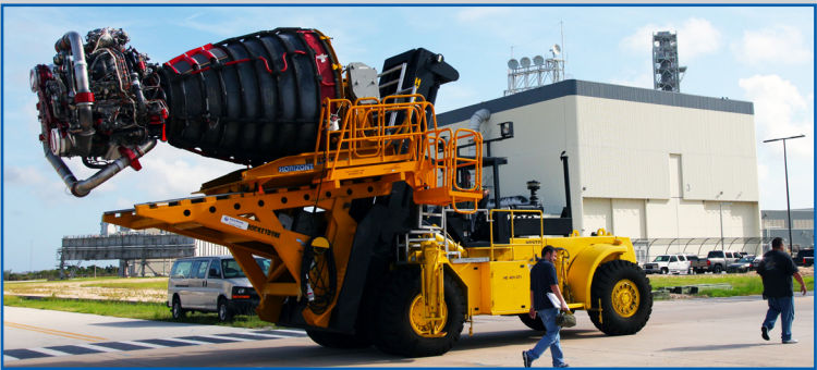
CLICK ON PHOTO NASA/Frankie Martin Technicians transport Engine No. 1, the final engine removed from space shuttle Atlantis, to the Engine Shop for possible future use Aug. 22. For more information, click on the photo.
