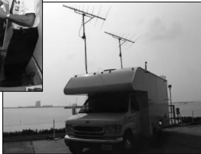
TOM Ruberto (above left) of Boeing and George Jenkins check out equipment in one of two specially equipped vans (exterior shown at right, parked at Static Test Road the day before the STS-85 launch). Each of the four radio receivers tracks a different commercial broadcast signal.
