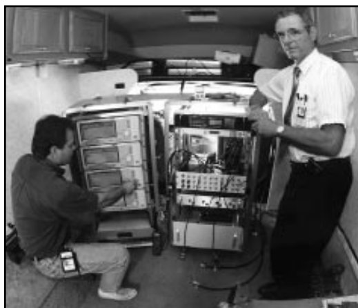
TOM Ruberto (above left) of Boeing and George Jenkins check out equipment in one of two specially equipped vans (exterior shown at right, parked at Static Test Road the day before the STS-85 launch). Each of the four radio receivers tracks a different commercial broadcast signal.
